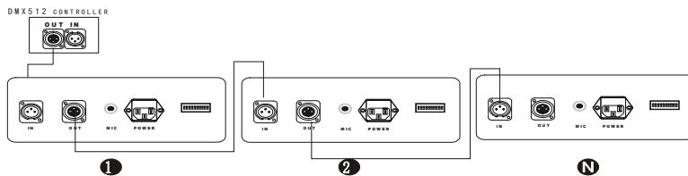
Note: Remember that the signal output port of the last luminaire is connected with a random attached circuit plug, which connects a resistance of about 120\_ between the 2 and 3 pins of the CANON (Caron Plug) plug. Connecting this circuit plug can effectively avoid noise and signal reflection during the transmission of the DMX512 signal.
